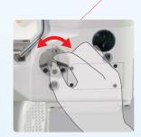
○The differential feed adjusting lever is located on the front face of the machine head.
