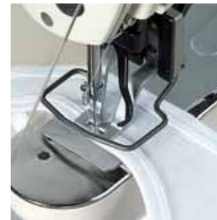
M type (Bartacking shoulder of running shirt)
